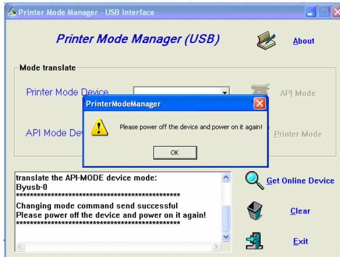
5. The printer mode manager should now have the AIP Mode button highlighted. (This indicates that the printer is now in the printer mode.) This is the correct mode for the printer to be in when it will be installed on a 64-bit PC.
