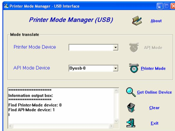
3. Select the correct printer in the *API Mode Device* field and click the **Printer Mode** button.
